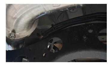
**Step 8. Installing the Y Pipe** Install the Y pipe.
